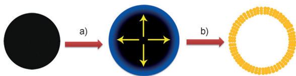
Figure 1. Illustration of the formation of \text{TiO}_2 hollow spheres using carbon spheres as templates: a) amorphous \text{TiO}_2 coating (blue) to form the \text{C@TiO}_2 core/shell structure; b) thermal annealing treatment to form polycrystalline \text{TiO}_2 hollow spheres (yellow).
